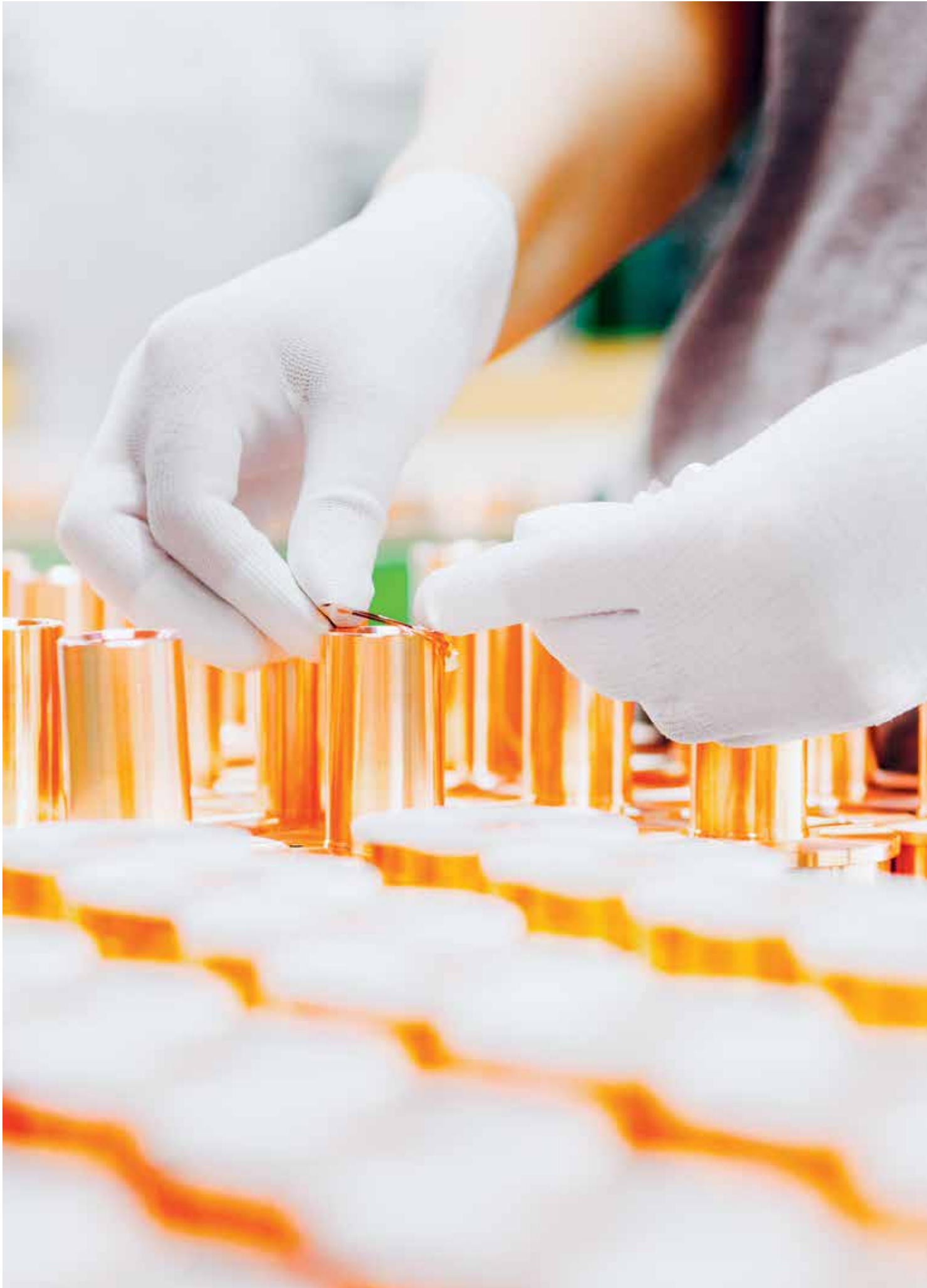
Assembling a vacuum capacitor.
