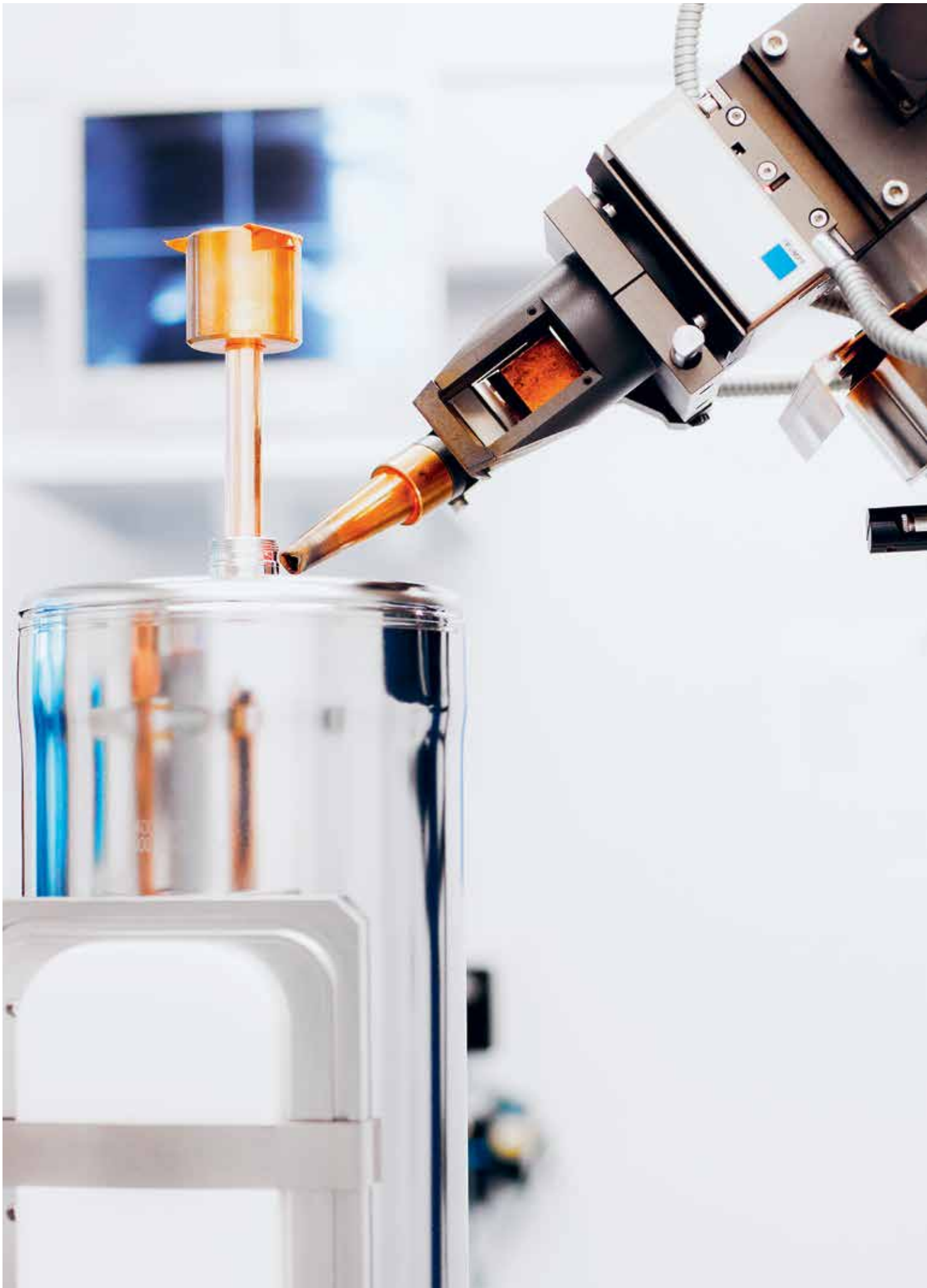
In the manufacturing of the ebeam lamps, ultra-high vacuum welds are achieved using the very latest laser welding technology.
