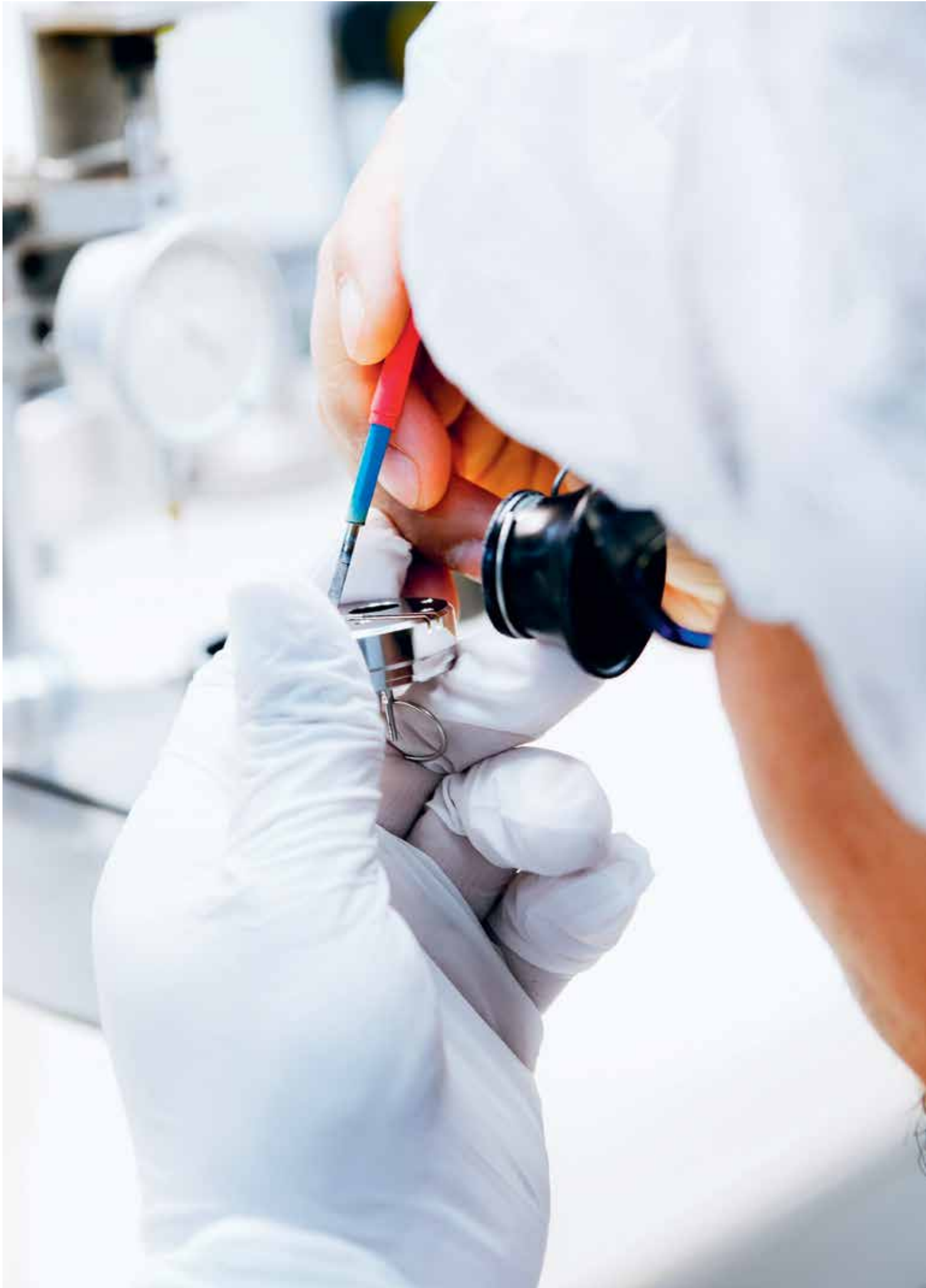
With a precision of up to one one-hundredth of a millimeter, a tungsten filament is aligned in a cathode.
