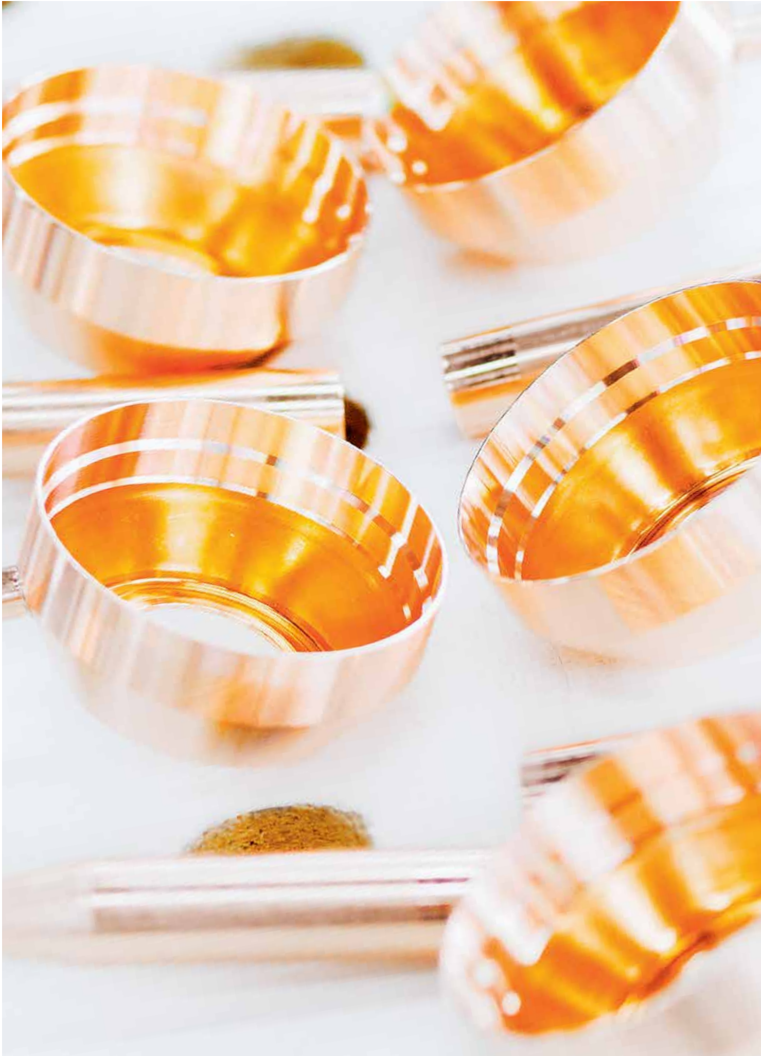
The copper parts of a vacuum capacitor, not yet plated with silver, are ready for assembly.
