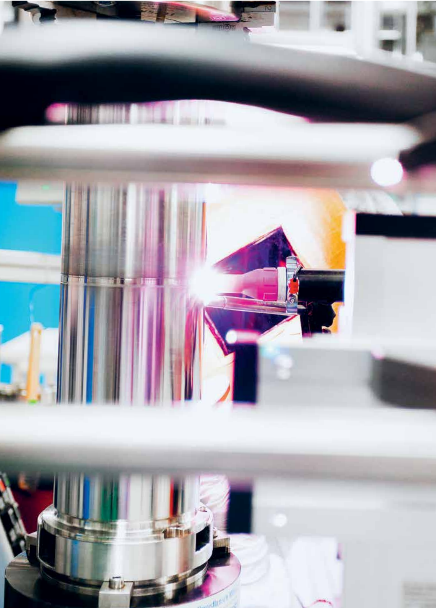
Only assembly in a climate-controlled environment can assure an ultra-high vacuum in the x-ray tubes.
